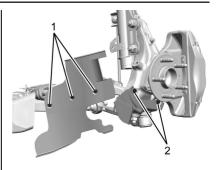
Install the small splash shields with two screws (2) per corner. Torque to 9 N•m (80 lb inch).
