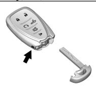
Press the button on the side of the RKE transmitter and pull the key out. Never pull the key out without pressing the button.
