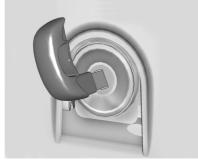
Remove any additional items attached to the key — such as keys, rings, or tags then fully insert the key into the manual release.
