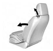
To access the rear seats, pull up on the latch on the top of the driver or front passenger seatback. Fold the seatback forward.
