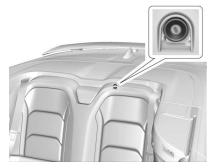
2. Locate the manual release beside the rear seat cushion on the driver side.
