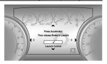
11. Auto Trans Only - Quickly apply full throttle. Release the brake pedal to launch the vehicle.
