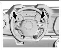
The sustem is activated and deactivated bu pressing either of the paddles marked REV MATCH on the steering wheel. The system must be activated with each new ignition cycle.
