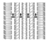
Treadwear indicators are one way to tell when it is time for new tires. Treadwear indicators appear when the tires have only 1.6 mm (1/16 in) or less of tread remaining. See *Tire Inspection* ⇒ 281 and *Tire Rotation* ⇒ 281 for additional information.
