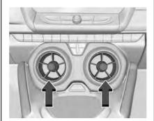
Use the air outlets in the center and on the side of the instrument panel to direct the airflow. Turn the center knobs on the air outlets clockwise or counterclockwise to open or close off the airflow.
