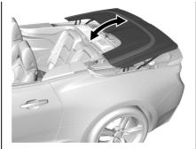
On each side of the tonneau cover, lift and pivot rearward into the fully open position. Hold the front and rear of the tonneau cover at the same time.
