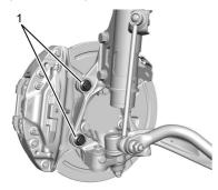
Apply liquid thread adhesive to the caliper bolts (GM Part No. 9985399 – Loctite 272 – Goodwrench 12345493).
