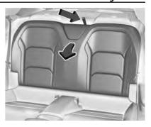
Pull the loop on the center of the rear seat back. The rear seat back will fold down.
