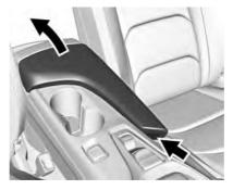
Press to open. If equipped, there are two USB ports and an auxiliary jack inside. See USB Port ⇒ 125 and Auxiliary Jack ⇒ 128.
