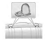
On coupe models, the top tether anchors are on the rear seatback filler panel.
